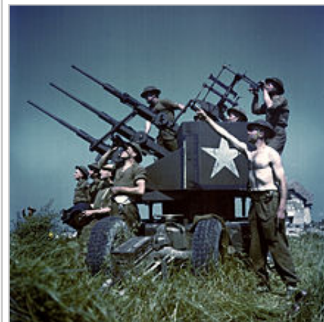
Anti-aircraft mounting, featuring three Polish Polsten cannons
